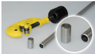
Result tube cutter (inside burr)
