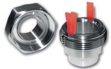
**ATTENTION: Remove the O-ring before you start the welding process, otherwise the heat will damage the O-ring.**
